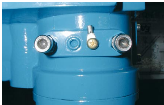
Fig. 6.5 -electrical installation - protective earth
